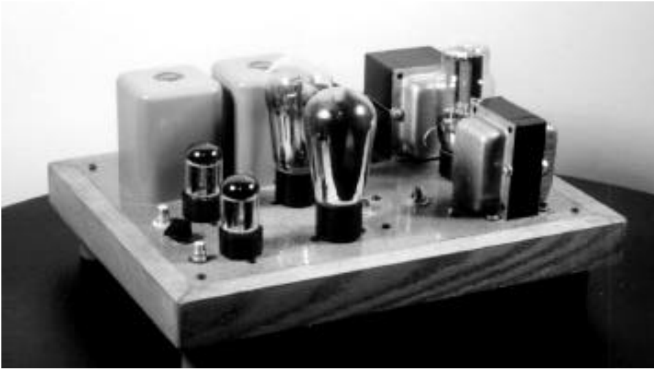
Globe 245 amp: Circuit is an SRPP 5691 with 2.2k,1W AB resistors,Facon .22uf paper in oil, 245 and a Tamura F475,5k OPTs. Kimber TCSS wire throughout.
